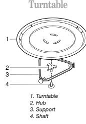
The turntable can rotate in either direction to help cook food more evenly. Do not operate the oven without the turntable in place. See "Assistance or Service" to reorder any of the parts.
